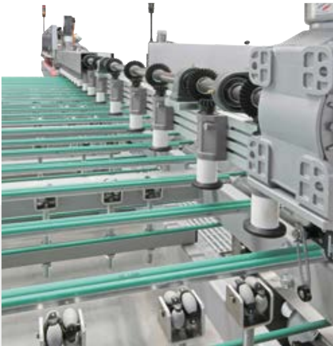
The passage from the upper surface to the belts is assisted by a pneumatic wheel system that avoids any type of damage to the glass.
