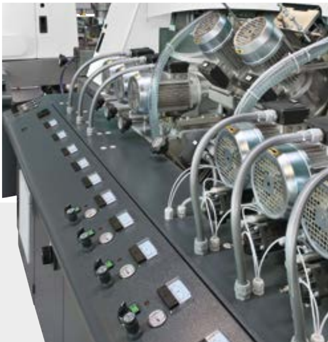
The ammeters to detect the current absorbed by the processing motors have been placed next to the corresponding spindles in order to facilitate readings by the operator engaged in adjusting the wheels.
