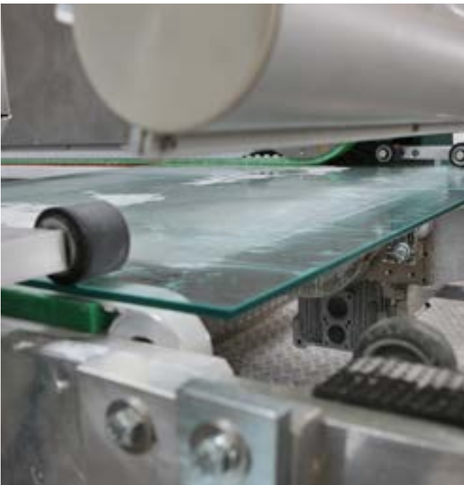
The air knives installed at machine exit, avoids contaminated water from the grinding process being transferred to the washing machine. This improves wash quality.
